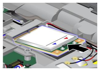
9. Pivot the card until you snap it into place. Secure the card with the screw.
